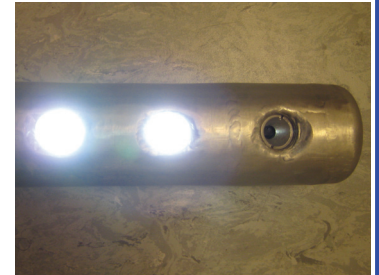
Two powerful LED lights seen in the water cooled camera. Only a 50mm large opening is needed for access.
